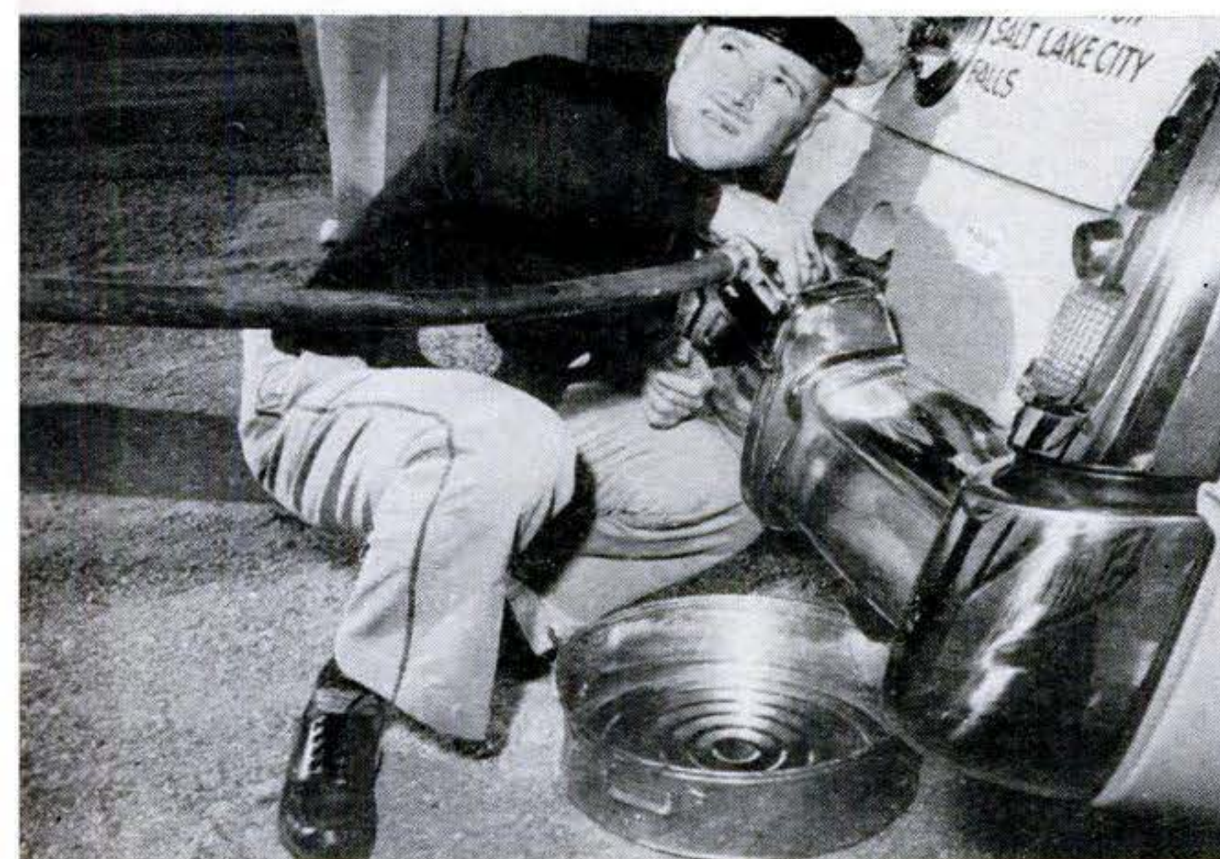
STATION ATTENDANT watches pump dial as he refuels a car at intermediate stop. Any gas spilled in pan was measured and deducted from total delivered to contesting car.
